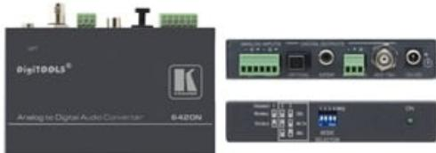
The 6420N is a high-performance format converter for balanced audio signals. The unit converts two channels of balanced audio signals to AES/EBU, AES-3id, S/PDIF and TOSLINK® optical digital outputs simultaneously
